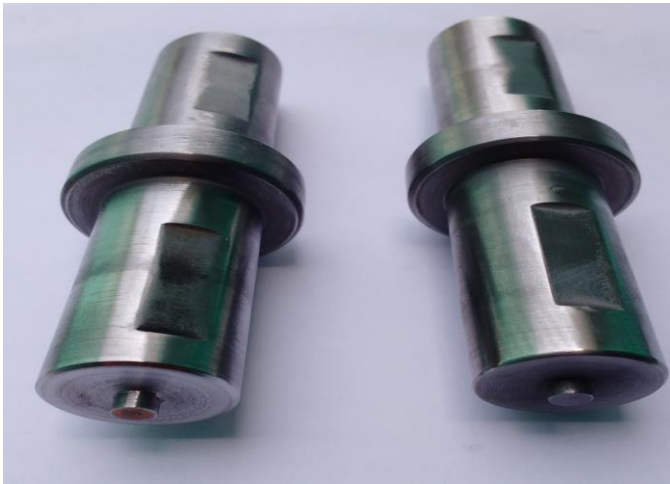
Figure 12 -FSW Tool –circular shape pin tool
