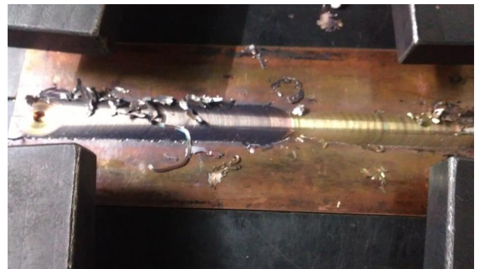
Figure 15 - Welded specimens after FSW
