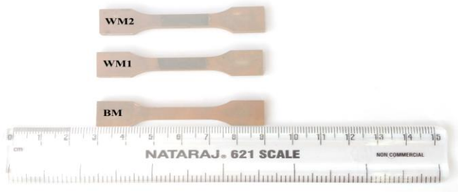
Figure 18 -Tensile Specimen Base Material 2&3. Welded Material
