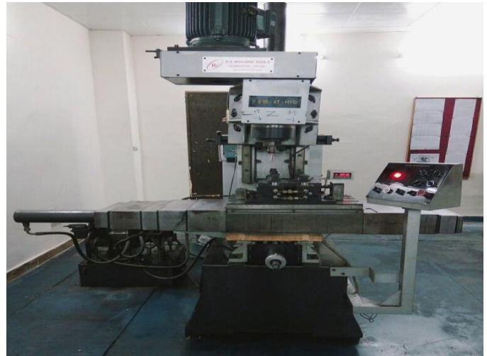
Figure 7 –Friction stir welding machine (DTU)
