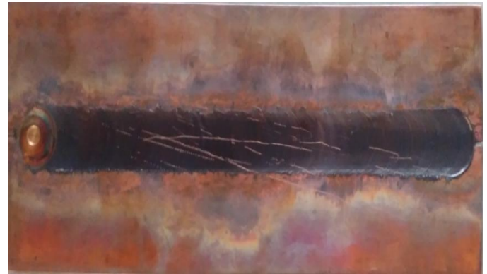
Figure 11 - Friction Stir Welded for \omega = 800 rpm and v = 60 mm/min, downward force= 7.5kN
