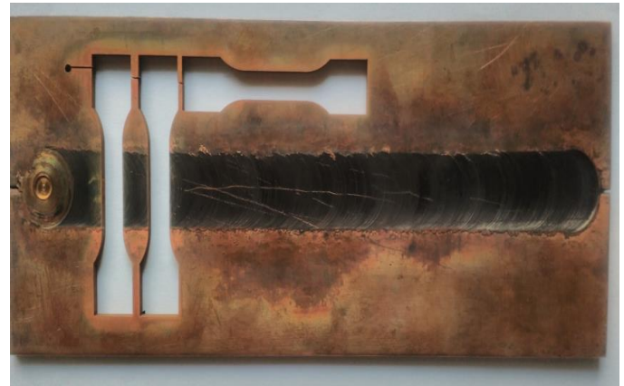
Figure 19 -Welded Plate after cutting Tensile Specimen
